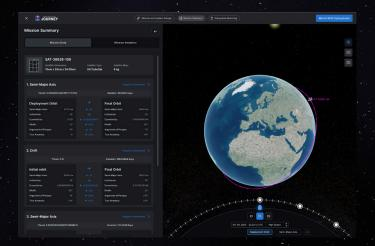
Mission Data outlines the Keplerian elements and their relative changes between a maneuver-specific initial orbit and final orbit. Additionally, it outputs the thrust required to perform this maneuver within the corresponding duration.
